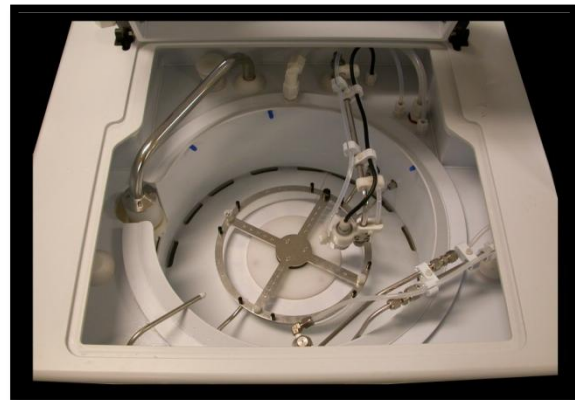
TYPICAL CLEANING CHAMBER & CHUCK (3 OF 4 ARMS SHOWN)
