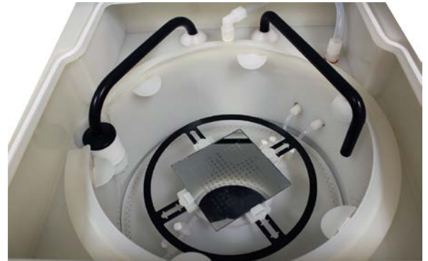
Example of Process Arms & 4"x4" to 9"x9" Adjustable Photomask Chuck
