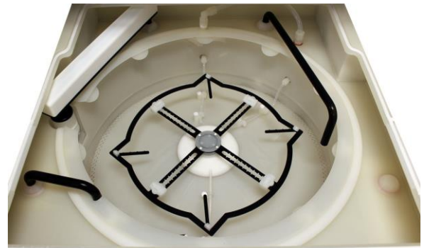
Example Process Chamber with 4"x4" to 14"x14" Photomask Adjustable Chuck
