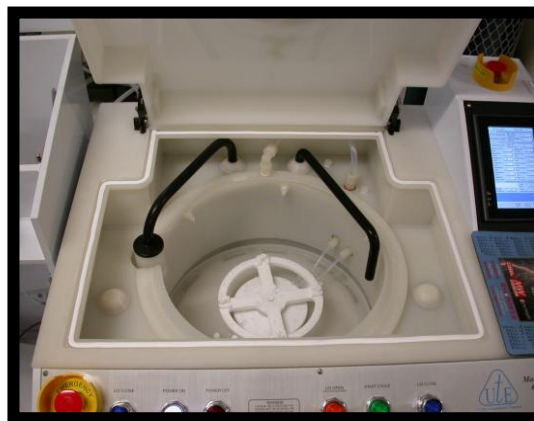
TYPICAL CLEANING CHAMBER & CHUCK
